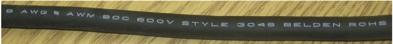
Wire markings showing incorrect 600V insulation rating.
